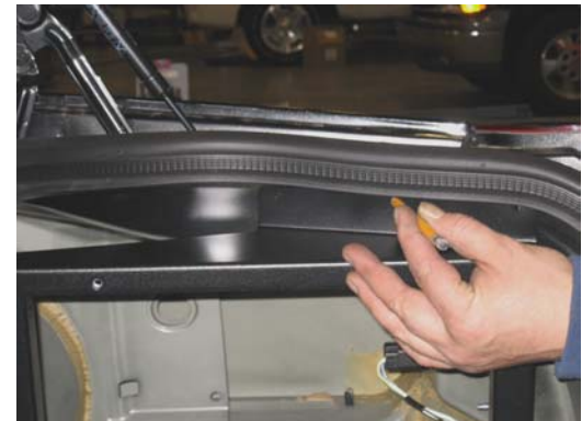
Position Trunk Side Mount and mark (3) holes on top mounting bracket
